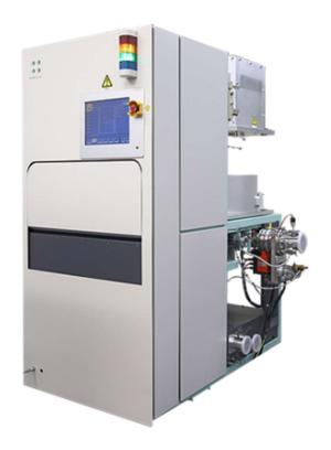
The Novellus Concept One and Two systems are proven PECVD workhorses in semiconductor wafer production, particularly for doped and undoped dielectric layers. First produced in the late 1980's, the C1 is a FAB mainstay with around 1000 systems still operating in the world today and has a batch load lock and "Sequel" chamber that performs batch PECVD deposition with an integrated clean step.
