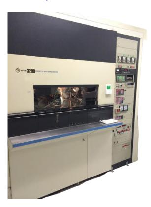
Varian launched the XM Series of PVD deposition systems in the late 70's, with the 3100 and 3200 series of vertical Sputtering coming later in the early 1980's. At Deptec we have many years experience on these toolsets and offer fully refurbished systems (sourced to order) and a whole host of upgrades to bring these systems into the technology and manufacturing practices of today's FABs.
